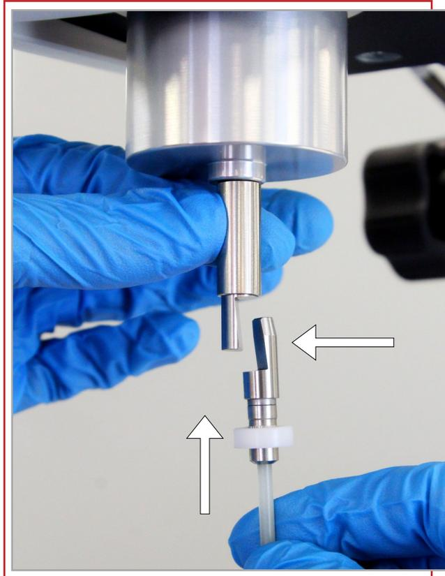
SimAir® Quick Connectors are included with the purchase of both the Scanning Brookfield PlusTwo (SB+2) D2983 Insert Module and the SimAir® Test Cell Assembly. The Coupling Top and Sleeve are provided with the module purchase, and the Coupling Bottom is included with the SimAir® Spindle. The design of the Quick-Connect spindle-coupling accessory allows the swift attachment or removal of the Spindle from the viscometer shaft.
