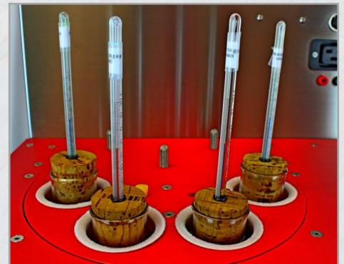
The SBT<sup>®</sup>+2 tests four (4) Cloud & Pour Point samples at a time. Accessories used with this Insert Module include Copper Sleeves, Glass Stators, Cork Rings & Discs, and Test Jar Stoppers.
