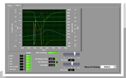
Auxiliary screens allow the user to set and view basic parameters, calibrate sensors, monitor real-time conditions, and perform diagnostics. The screen depicted here contains a graph that is generated in real time during a test, enabling the user to troubleshoot various problems, such as evaluating whether an injector nozzle needs maintenance, determining whether a sensor or cable is malfunctioning, and ensuring appropriate combustion. The user can choose which sensor signals are displayed.
